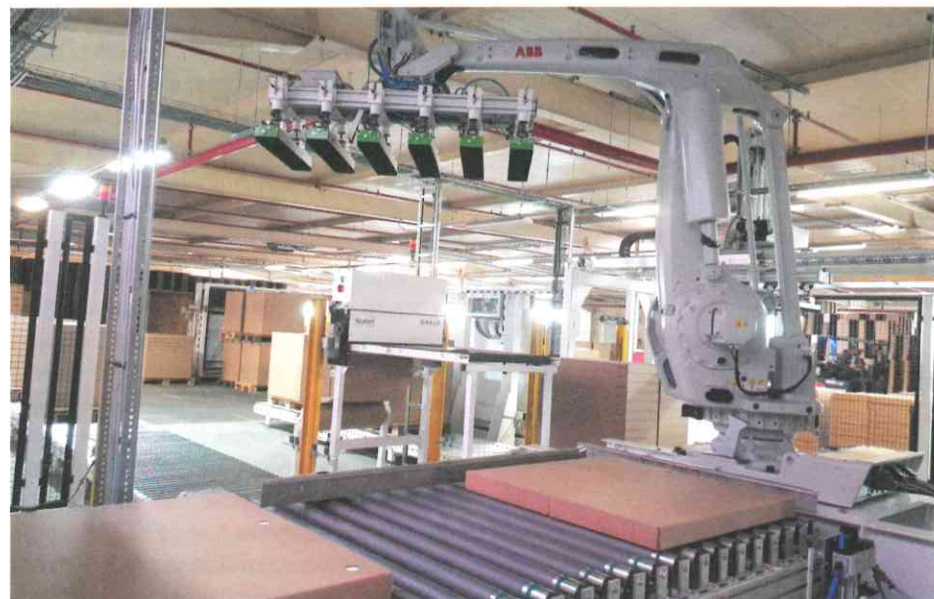
The furniture parts are placed on the existing layer on the pallet.
