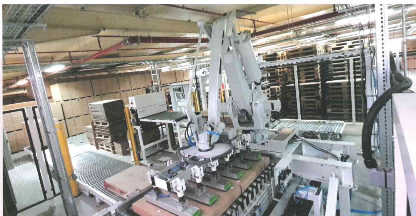
The robot, which is also equipped with an EOAT consisting of six Kenos® KVG area grippers from Piab, picks up a layer of furniture parts packed in boxes from the roller belt.
