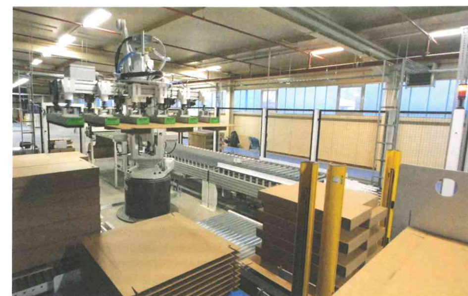
The robot with the EOAT made of Kenos® KVG area grippers picks up a cardboard pallet.
